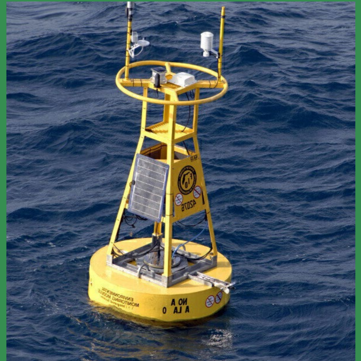
Data Collection Buoy, CARICOM Climate Change Centre partners with global institutions to deploy the integrated buoy network
