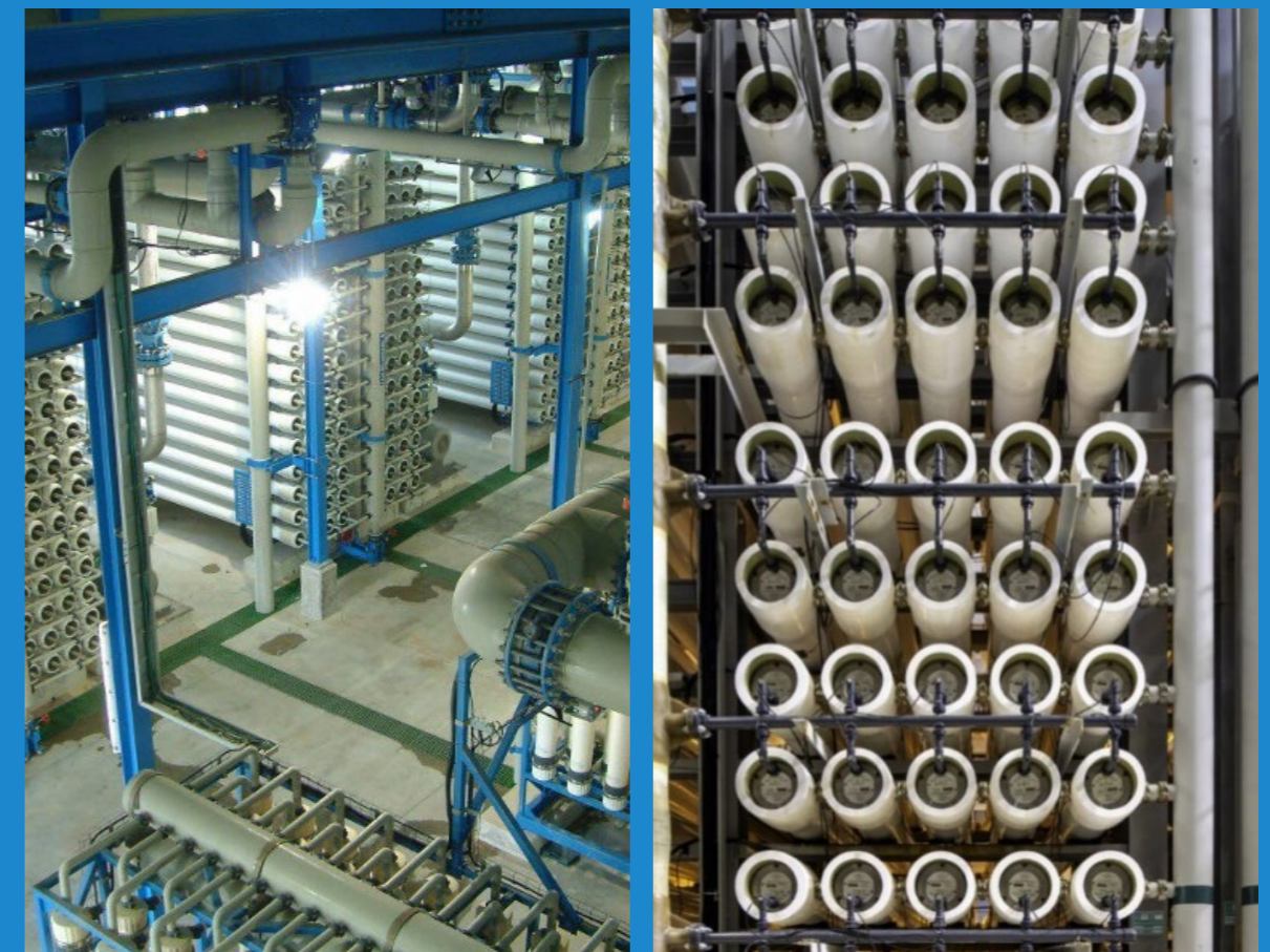
Reverse osmosis equipment inside a saline water desalination plant, Saline Water Conversion Corporation
